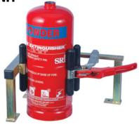
This manual clamping machine is adjustable for all sizes of fire extinguisher. Fire extinguisher can be secure firmly when opening or tightening valve on the cylinder.
