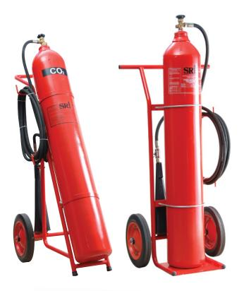
Carbon dioxide fire extinguisher on trolley is made of seamless Manganese steel to withstand high storage pressure. It is effective on class B and class C fires and electrically non conductive.
