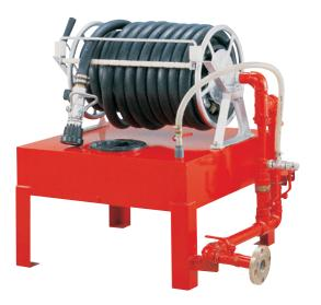
This hose reel station is complete with 1-1/2" x 30M rigid hose, 120L AFFF foam, stainless steel foam concentrate storage tank, 95GPM foam inductor and nozzle. A bypass loop is provided for water or foam discharge.
