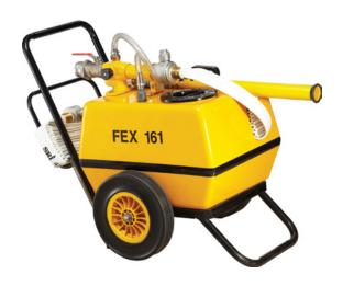
The foam liquid extinguisher on trolley is highly manoeuvrable and it is suitable for outbreaks of fire that cannot be dealt with by using portable extinguishers. It is effective on flammable liquid fire. This is a self-contained foam production unit which only requires connection to suitable water supply (minimum water supply required is 180 LPM at 5 bar).
